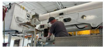
The most challenging part of my job is diagnosing and resolving emissions problems as they can be misleading and tricky to solve. We deal with emissions issues because the trucks sit and are run for the hydraulics, which gums them up as they don't generate the heat needed to burn off the particulates.
